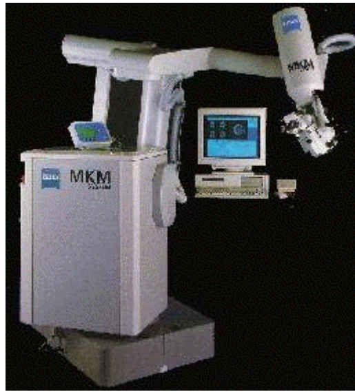
The Zeiss MKM Microscope transport. It is a 6-degree of freedom robot with a surgical stereomicroscope attached.
